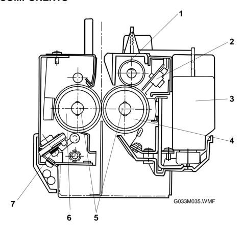
1. Cleaning Roller Cleans the hot roller.
