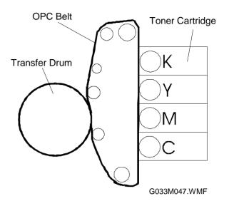
2) The developed toner images are transferred to the transfer drum one at a time (a).
